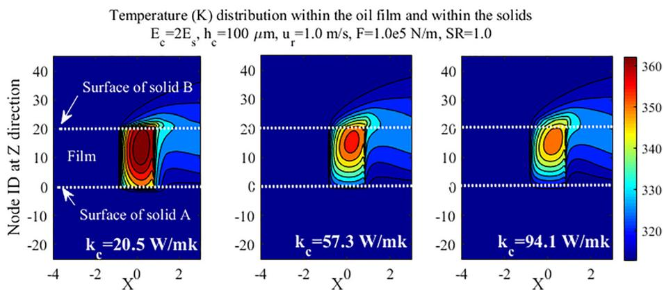
Fig. 5 Temperature distribution under three thermal conductivities of the coating
