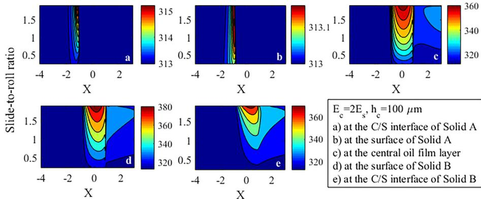
**Fig. 2 Effect of slide-to-roll ratio on temperature profile at five characteristic layers**
