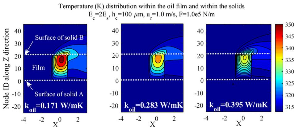
Fig. 6 Effect of the thermal conductivity of the fluid on temperature distribution
