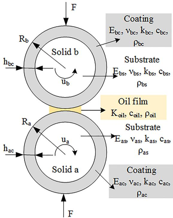
Fig. 1 The lubricated contact between two coated rollers
