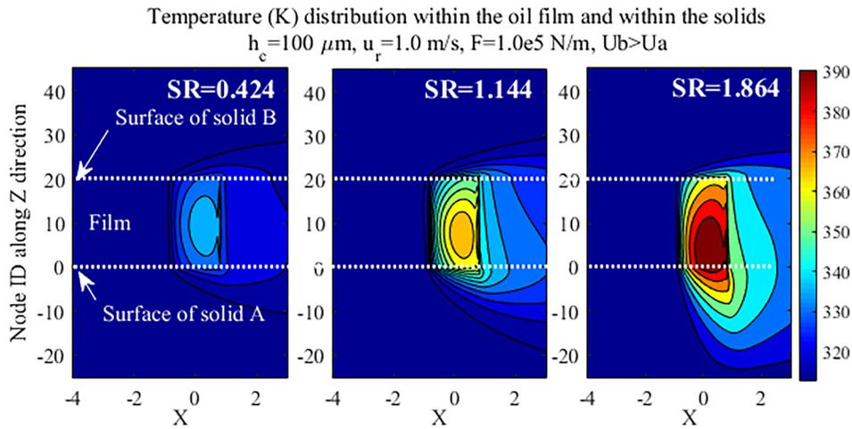
Fig. 4 The temperature distribution under three slide-to-roll ratio cases with  $u_b>u_a$
