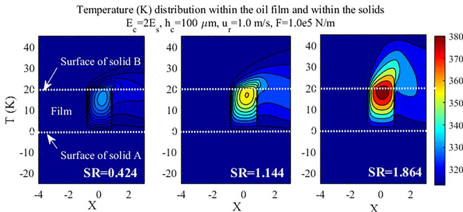
**Fig. 3 The temperature distribution under three slide-to-roll ratio cases**
